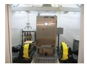
VeloDyne's MAKO  $^{\rm M}$  HDL Slurry System utilizing weight and density controll and monitoring.
