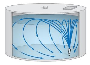
The PAX Water Mixer creates a powerful vortex flow pattern to thoroughly mix the entire tank volume.
