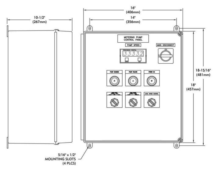
Enclosure Rating: NEMA 4X, Fiberglass Power
