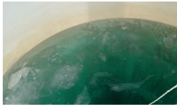
Figure 3b. Ice conditions inside the tank after 24 hours of mixer operation. The ice has substantially melted and open water is visible in many areas.
