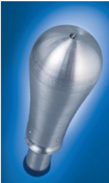
Figure 2. The PAX Water Mixer (PWM100) for small tanks. The vortex mixer is 30 inches tall, weighs 40 pounds and can be self-installed.
