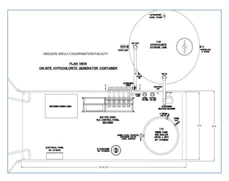
Thanks to the containerized Microclor® OSHG system, LADWP's Mission Wells chlorination facility has a safe and reliable source of chemical disinfection that has simplified operations. This system continues to operate to this day.
