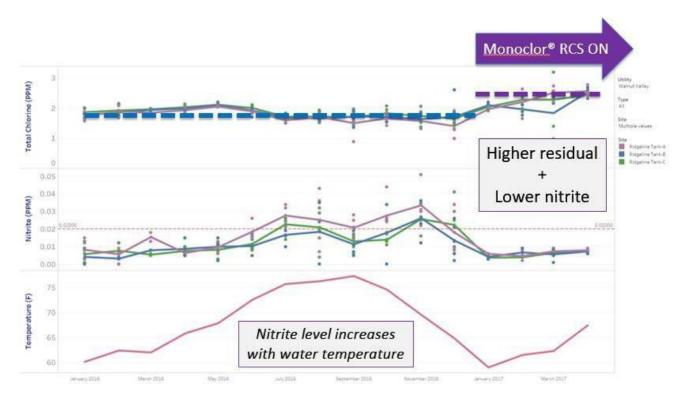
With the implementation of the PAX/PSI Monoclor® RCS system, Walnut Valley was able to reduce the nitrite (nitrification precursor) levels as well as improve residual levels in the service area. The elimination of energy intensive deep tank cycling was a bonus as was the elimination of the labor intensive practice of breakpoint chlorination.
