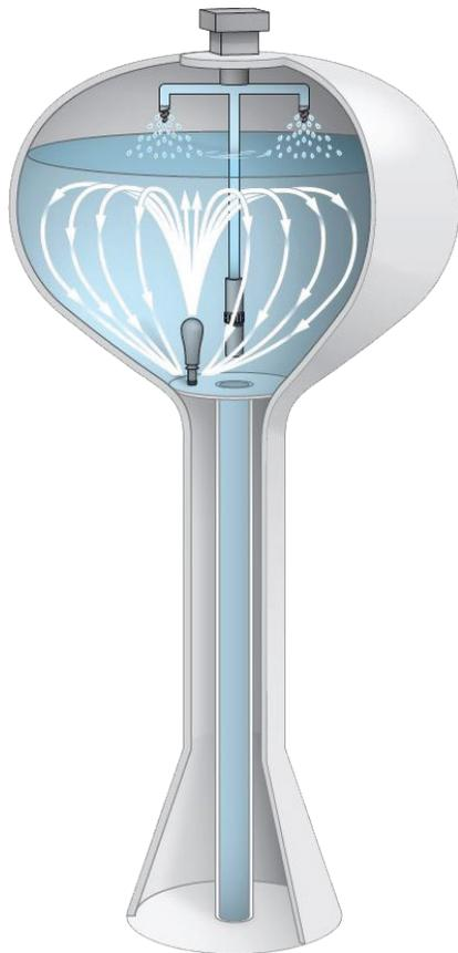
Active mixing and ventilation are the first steps in THM removal. The PAX Mixer continually introduces THM-concentrated water to the surface where THMs are volatilized and evacuated.
