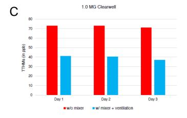
THM reductions measured on 3 different days in the Colfax water system. Average THM removal rates were 45% for the 1.0 MG and 0.3 MG clearwell tanks and 65% for the 0.6 MG Ballpark Tank
