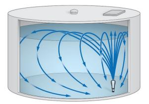
The PAX Water Mixer creates a powerful vortex flow pattern to thoroughly mix the entire tank volume.
